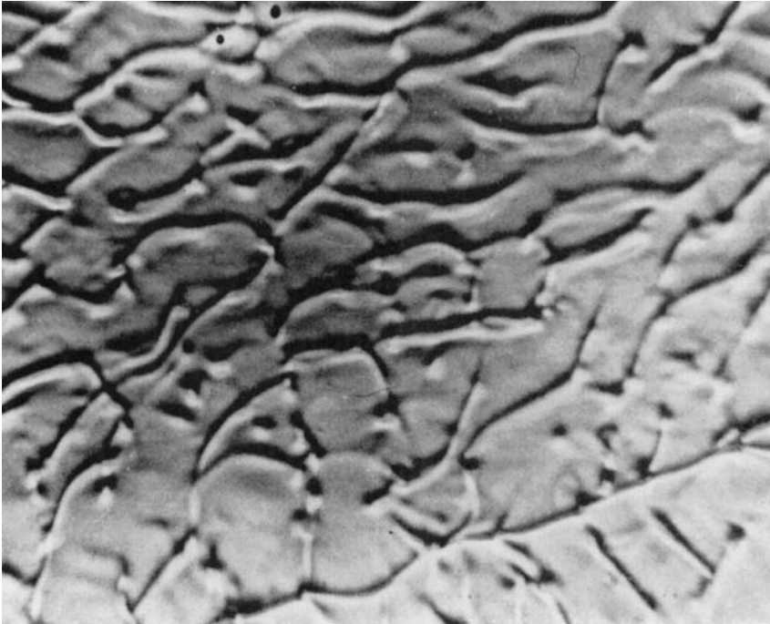
FIGURE 20. Water desorbing from a 10 mm deep pool composed of equal volumes of water and 1,4-dioxane. Magnification 1·8.
