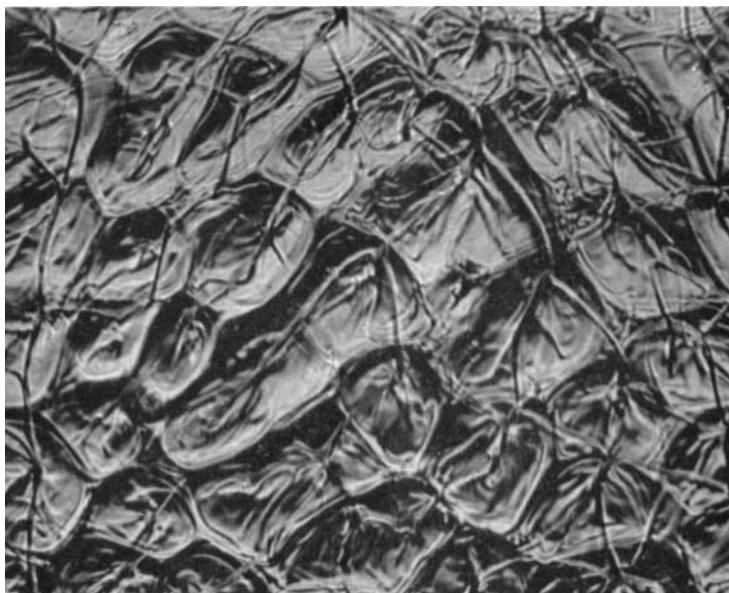
FIGURE 23. Benzene desorbing from a 6 mm deep pool composed of equal volumes of benzene and a silicone oil (Dow Corning Fluid 200-50). The system is subject only to buoyancy-driven convection. Magnification 1.8.
