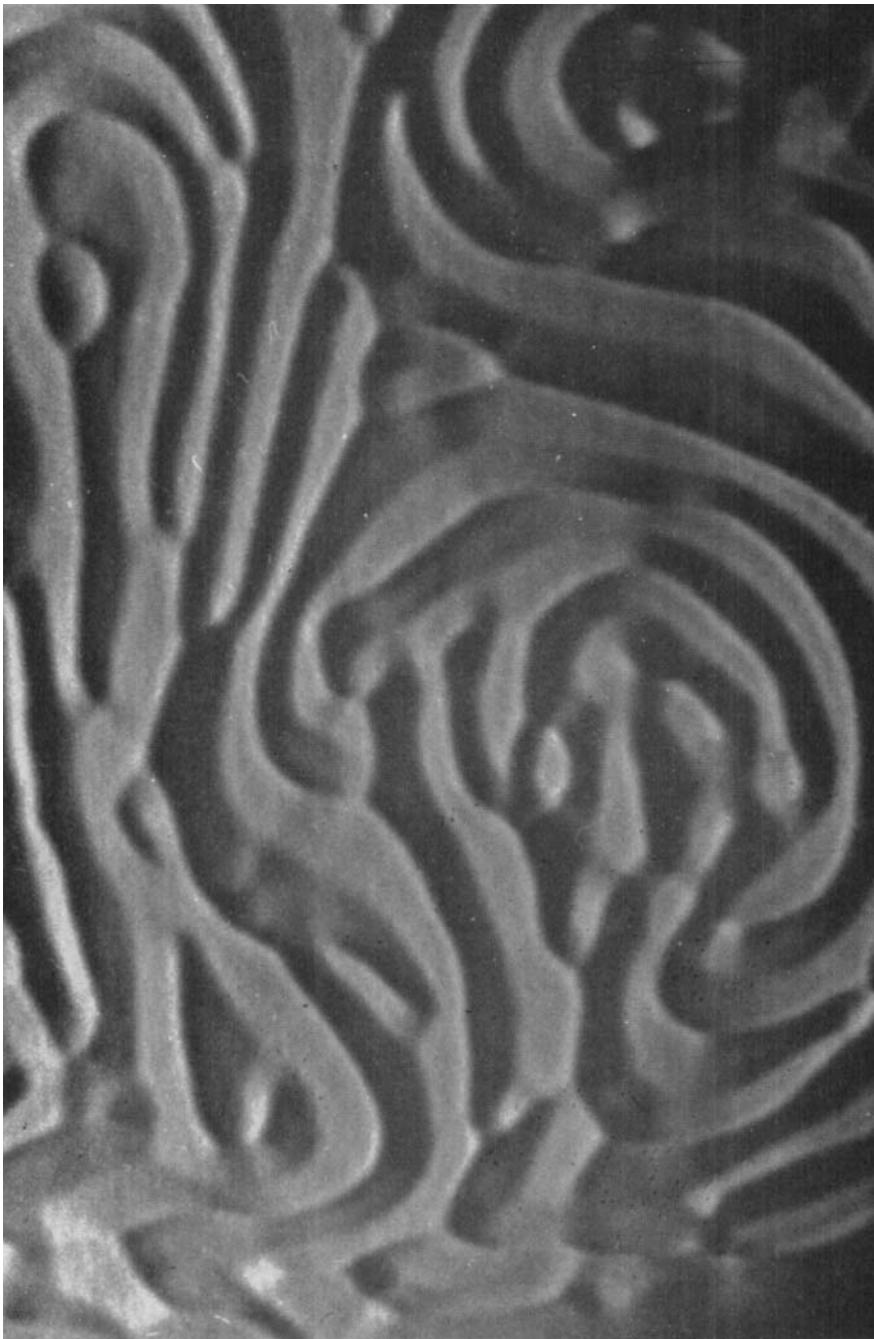
FIGURE 14. Vermiculated roll cells in a 3 mm deep pool of carbon tetrachloride. Surface is contaminated with a trace amount of paraffin wax. Magnification 3·5.
