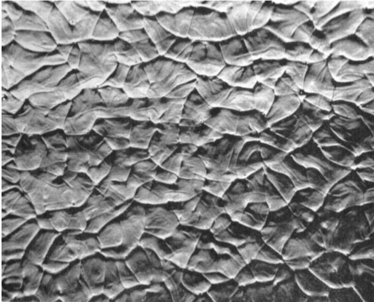
FIGURE 21. Acetone desorbing from a 7 mm deep pool composed of equal volumes of acetone and carbon tetrachloride.
